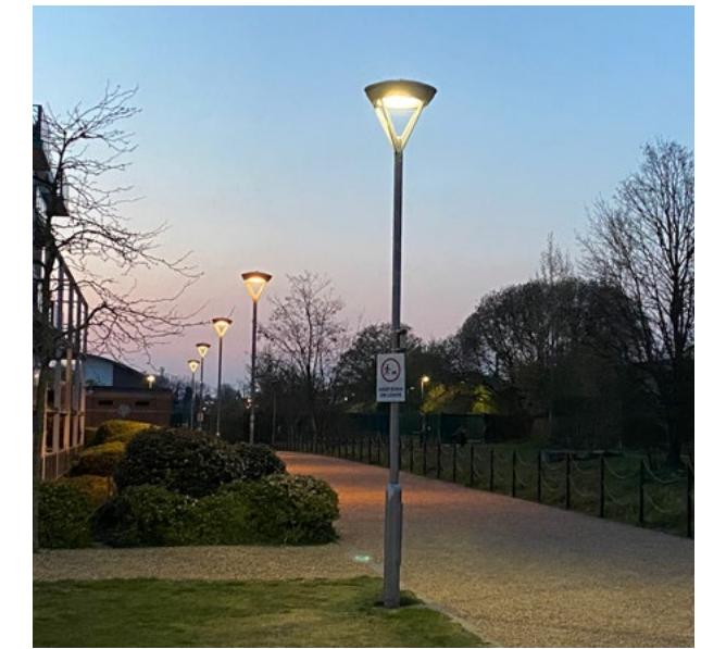
Pedestrian level lighting using low luminance to minimise impact on adjacent wildlife corridor
