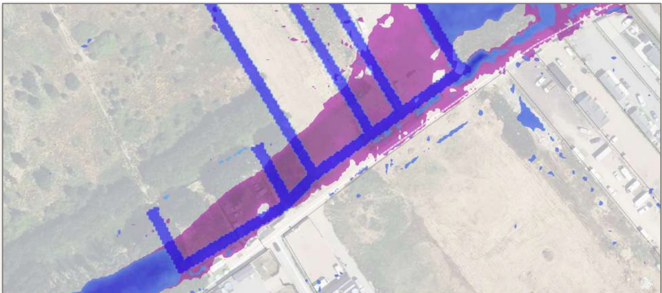
FIGURE 16 – MODELLED SURFACE WATER FLOOD EXTENT AT ACCESS ROUTE, PRE (PURPLE) AND POST-DEVELOPMENT (BLUE) DESIGN EVENT
