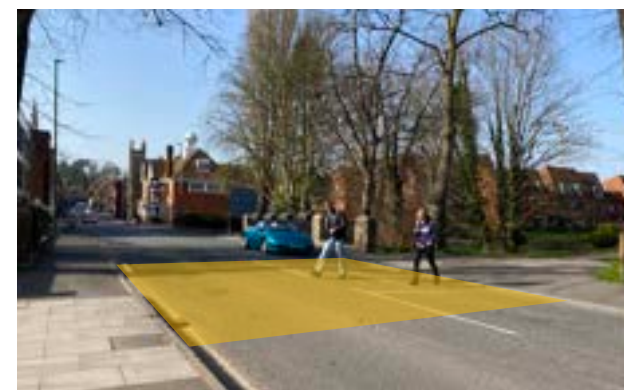
Figure 77. Indicative location (highlighted in orange) for a raised table to facilitate pedestrian crossings between Borelli Walk and Gostrey Meadow, and connections for people cycling between Borelli walk and proposed cycle facilities to/from Station Hill (proposal #4)
