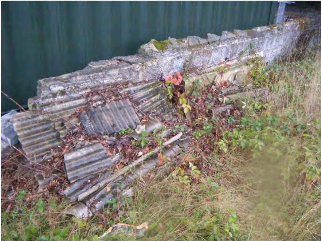
Plate 15: Image showing the small pile of corrugated asbestos cement sheets and fragments present beside the shipping containers in the centre west of the site.
